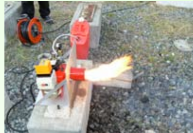
Burner combustion experiment using recycled oil
