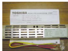
Inverter/VFD type fluorescent lights
