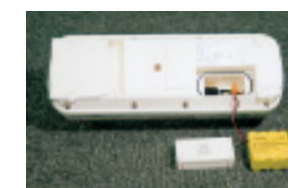
Removal of syringe pump rechargeable batteries
